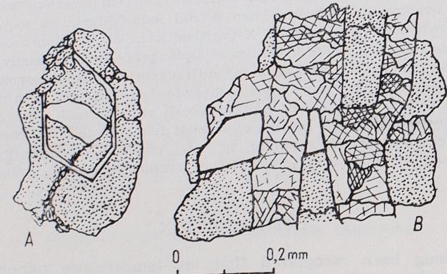
Fig. 1. Quartz crystal forming euhedral perymorph around small detrital quartz nucleus in a micrite of pseudoolite limestone from Lipowa (A).
