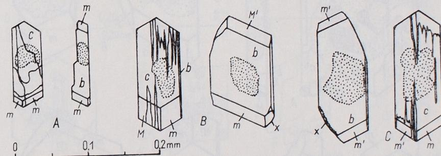
Fig. 2. Predominant shapes and habits of authigenic (epitaxial) albite grains in Cieszyn limestone from Lipowa and Žywiec localities. Doubly positioned crystal sketches display X-Carlsbad (grain A) and albite twin-law (grain B and C) structures. Spotted areas indicate relict (detrital) soda-feldspar nuclei. Faces labelled after Dana nomenclature;  $x$  = irrational surfaces
