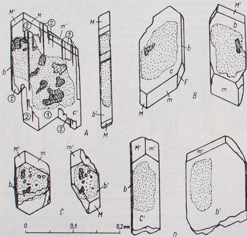
Fig. 3. Aberrant shapes and habits of authigenic albite grains from the same occurrences. The only twinned grain (A) shows albite- and possibly X-Carlsbad rule of twinning
