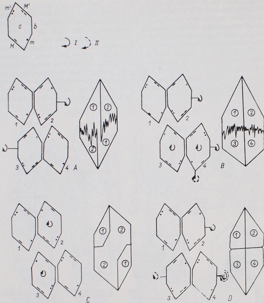
Fig. 5. Schematic presentation of plagioclase crystal fourlings twinned after albite (A), Roc Tourné (B), Carlsbad (C), and X-Carlsbad (D) twin laws and their origin. Note the rectilinear composition surfaces and parallelity of net planes in opposite quadrants of Carlsbad twins. Numbers denote the sequence of twinning operations and those in circles — subindividuals with separate lattice orientation; I — rotation, II — second kind rotation.
